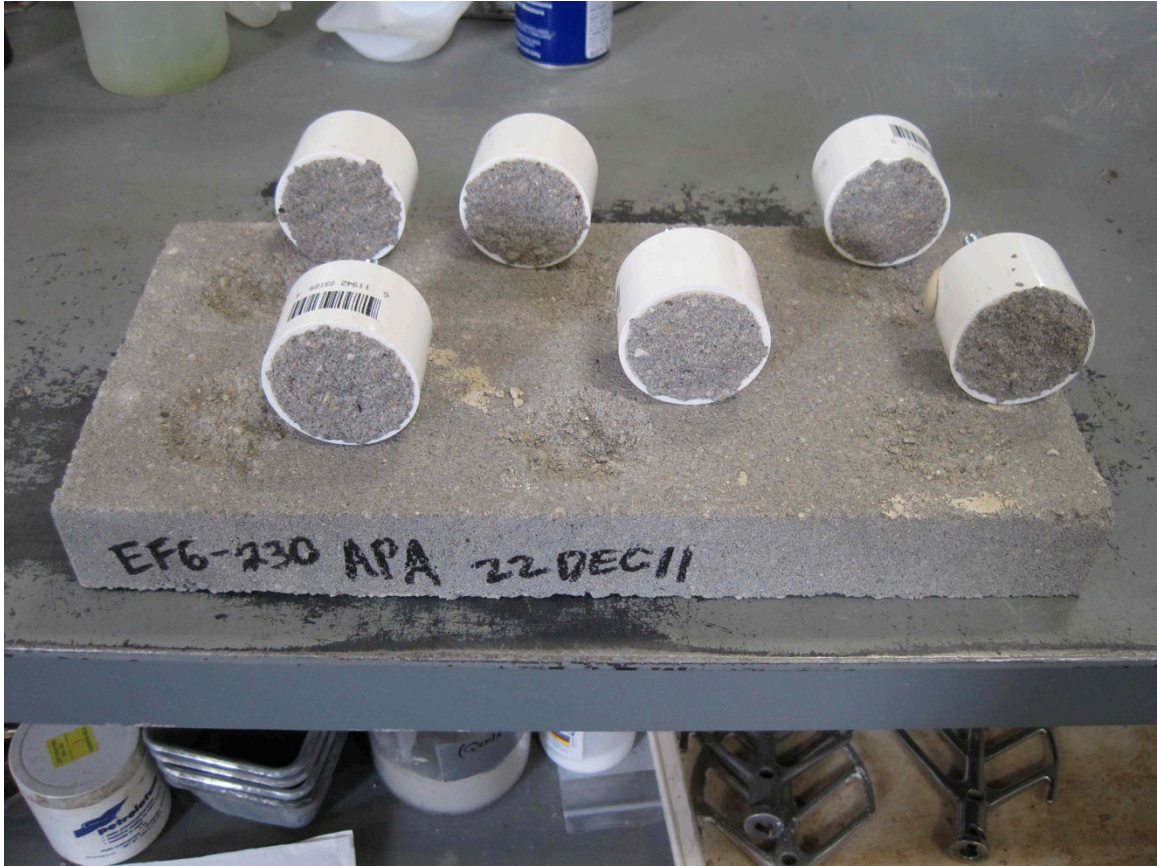
Figure 6.1.13: CSA cement mortar 1 plus polymer 1 displaying failure mode CF/S, substrate failure, following pull-off testing over concrete substrate 2 after curing for 13 days at ambient laboratory conditions
