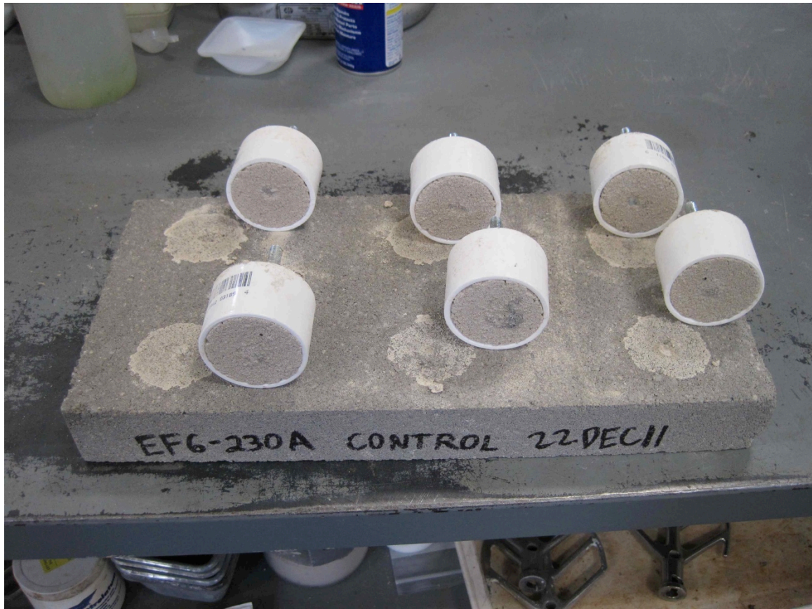
Figure 6.1.12: CSA cement mortar 1 displaying failure mode AF/S following pull-off testing over concrete substrate 2 after curing for 13 days at ambient laboratory conditions
