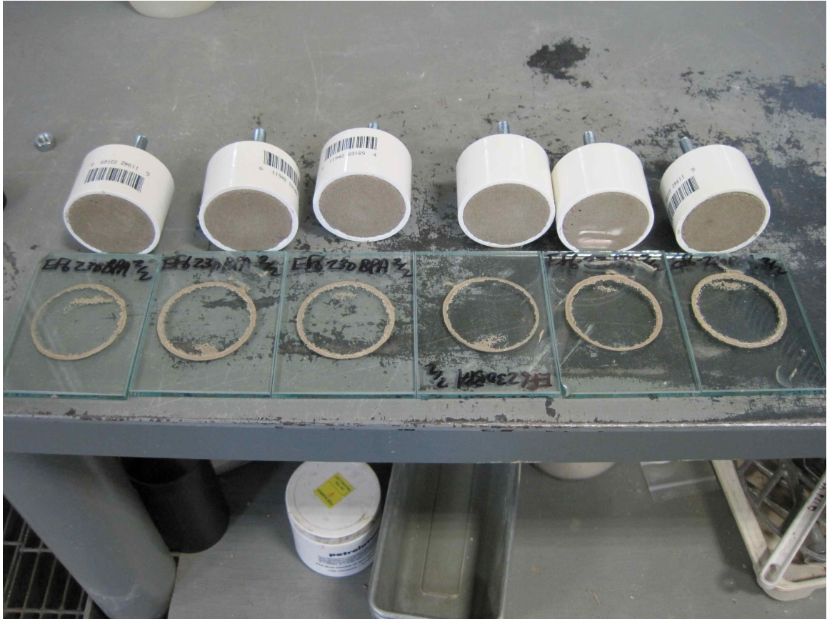
Figure 6.1.15: CSA cement mortar 1 plus polymer 2 with p/c = 0.15 displaying failure mode AF/S, failure at bond line, following pull-off testing over glass substrate after curing for 7 days at ambient laboratory conditions
