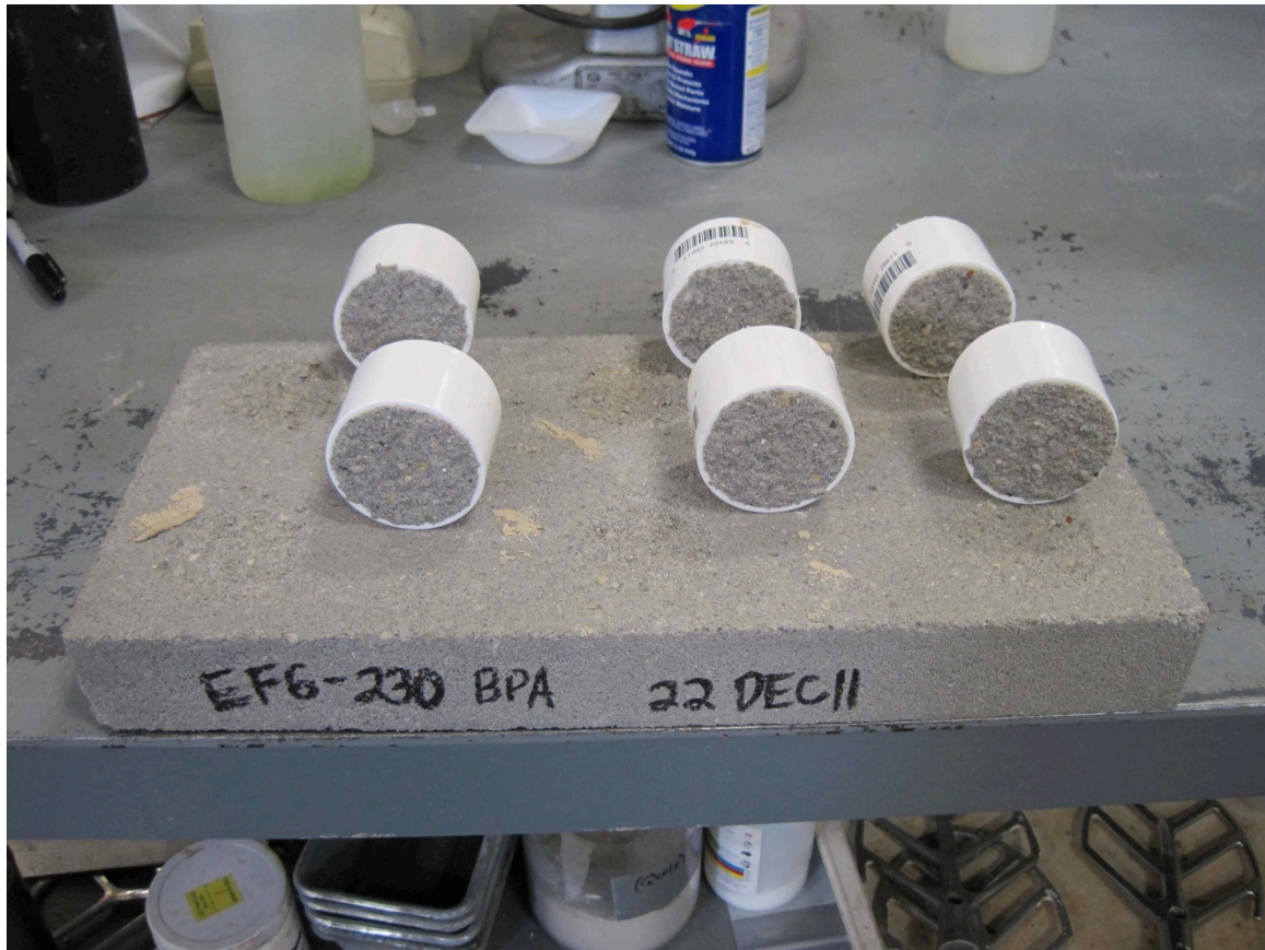
Figure 6.1.14: CSA cement mortar 1 plus polymer 2 displaying failure mode CF/S, substrate failure, following pull-off testing over concrete substrate 2 after curing for 13 days at ambient laboratory conditions
