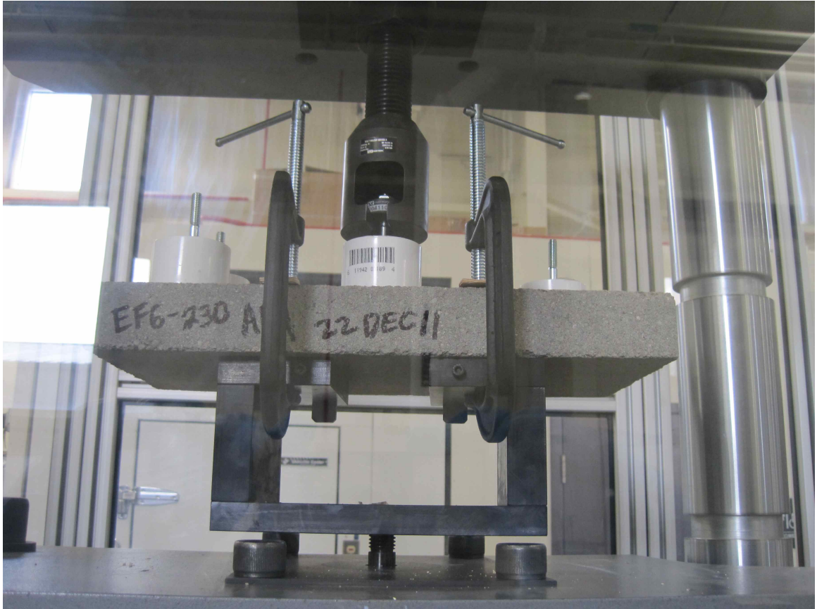
Figure 6.1.2: This figure illustrates “pull off” testing in progress utilizing an Instron universal testing machine
