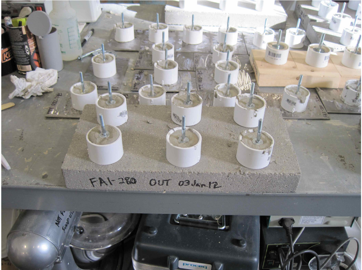
Figure 6.1.1: Adhesion test specimens cast over various substrate materials with concrete in the foreground while ground metal and wooden substrates can be seen in the background
