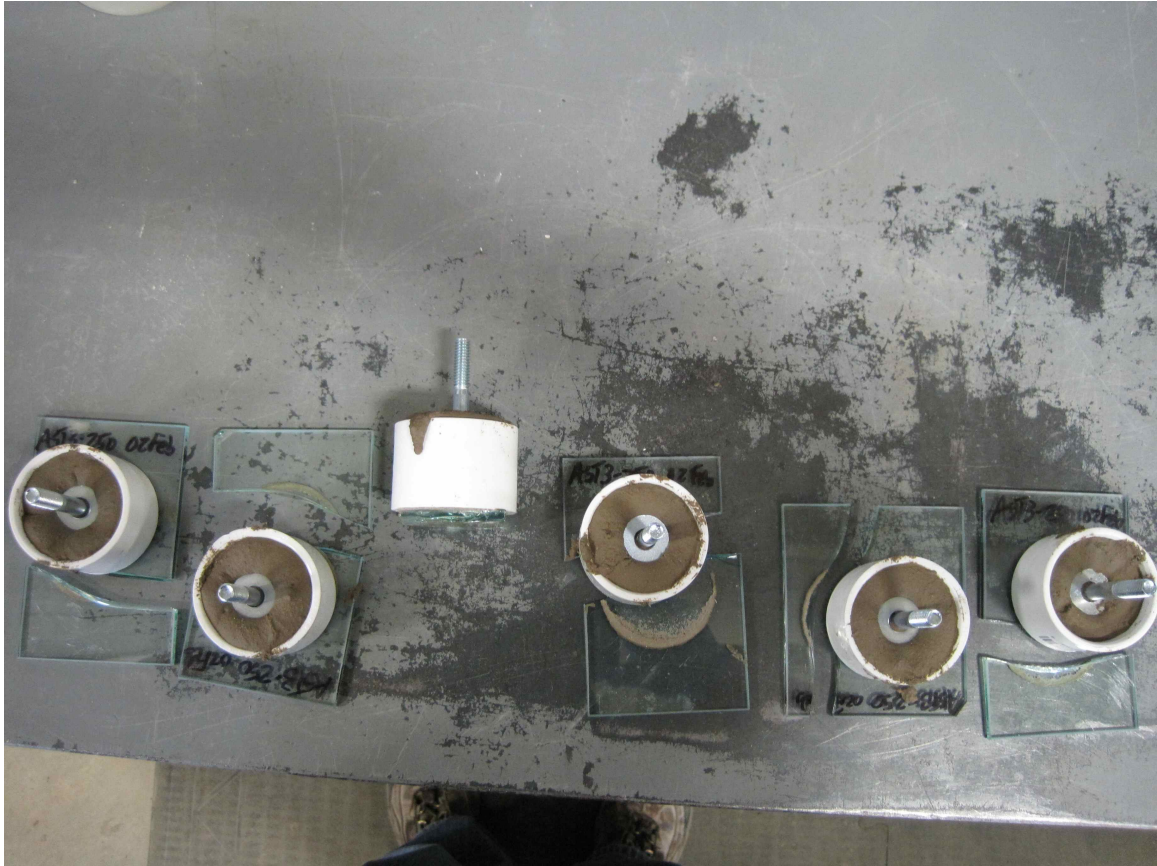
Figure 6.1.17: CSA cement mortar 1 plus polymer 2 with p/c = 0.45 displaying failure mode CF/S, substrate failure, following pull-off testing over glass substrate after curing for 7 days at ambient laboratory conditions.
