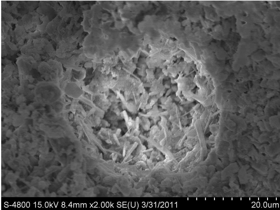
Figure 5.3.11: SEM image of control CSA cement paste listed in Table 5.3.2 after curing for 7 days at 50% relative humidity and 23°C
